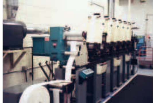
An Enercon XL treater on Comco Press at Fox Valley Technical Collage.
