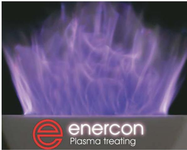
Blown-arc air plasma is formed by blowing atmospheric air past two high-voltage powered electrodes and is sometimes referred to as corona treatment.
