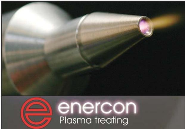
Blown-ion air plasma systems push pressurized air past a single electrode which discharges inside the treater head. The electrode creates positively charged ions in the surrounding air particles. The air pressure forces the air particles to accelerate out of the tip of the head as a high-velocity stream of charged ions directed toward the substrate surface.
